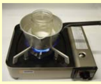
Figure 1. Flash-heat experiment using simple equipment (same equipment used for Pretoria Pasteurization)
